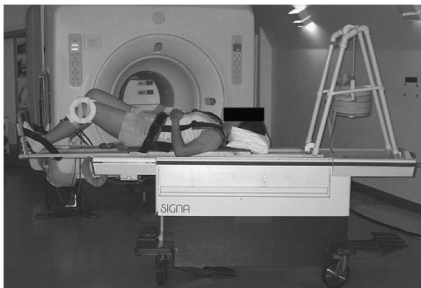
Fig. 1. Custom non-ferromagnetic leg press (Captain Plastic, Shoreline, WA) used to simulate weight-bearing. A resistance of 25% body weight was used to load the knee extensor mechanism. Reprinted with Permission from Salsich GB, Ward SR, Terk MR, Powers CM. In vivo Assessment of Patellofemoral Joint Contact Area in Individuals Who Are Pain Free. Clin Orthop 417, 277–284, 2003.
